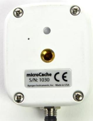
A sensor's model number and serial number are located on the back of the  $\mu$ Cache unit. If you need the manufacturing date of your  $\mu$ Cache, please contact Apogee Instruments with the serial number of your  $\mu$ Cache.
