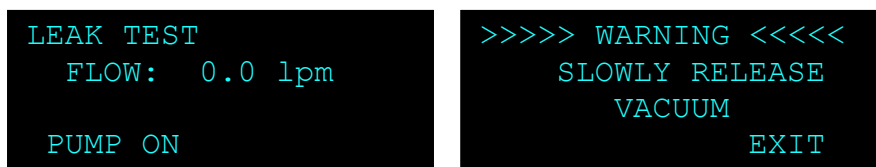
Figure 7-10 The C-12 Leak Test Menu
