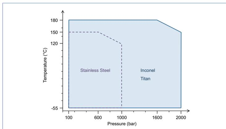
KELLER 7LHP series high pressure transducers are available with various material options. Stainless steel, Inconel 718 or titanium can be selected (see "Mechanical data") in line with requirements.
