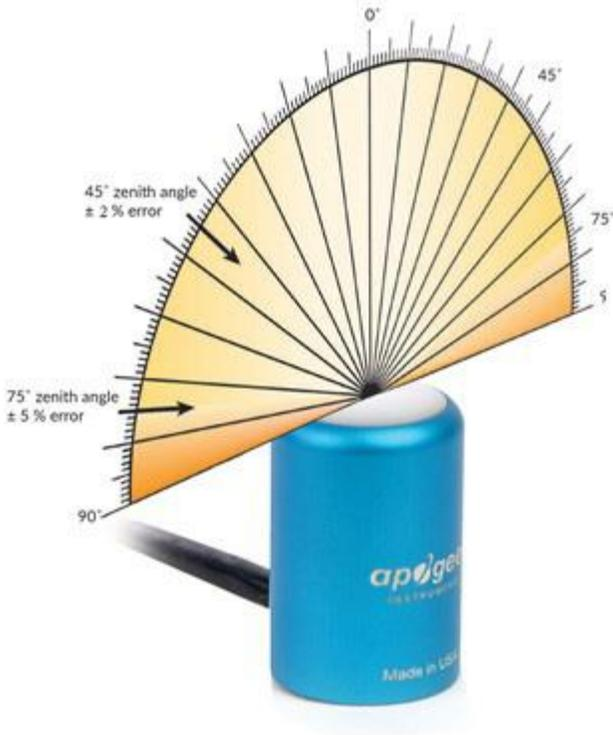
Directional (cosine) response is defined as the measurement error at a specific angle of radiation incidence. Error for Apogee MQ-500 series quantum sensors is approximately  $\pm 2\%$  and  $\pm 5\%$  at solar zenith angles of 45° and 75°, respectively.
