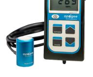
Research-grade measurements of underwater photosynthetically active radiation
