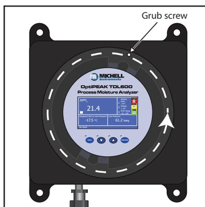
4. Remove the blue, circular display PCB by undoing the two Panax fasteners located on the display mounting brackets.
