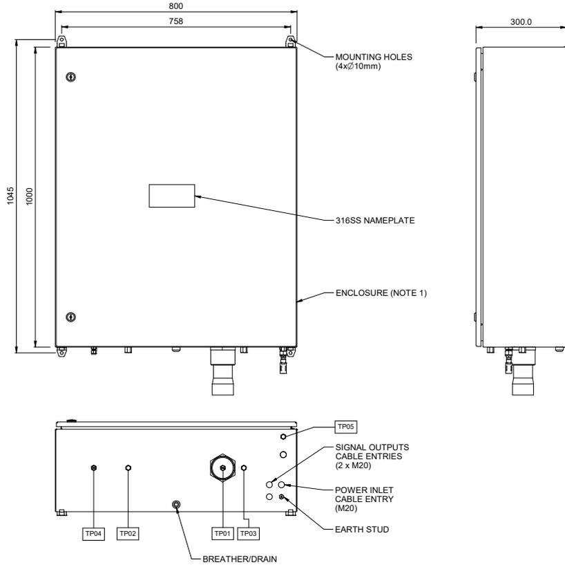
Figure 34 Dimensional Drawing – Outdoor System Enclosure
