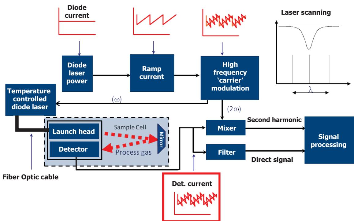
Figure 3 System Block Schematic
