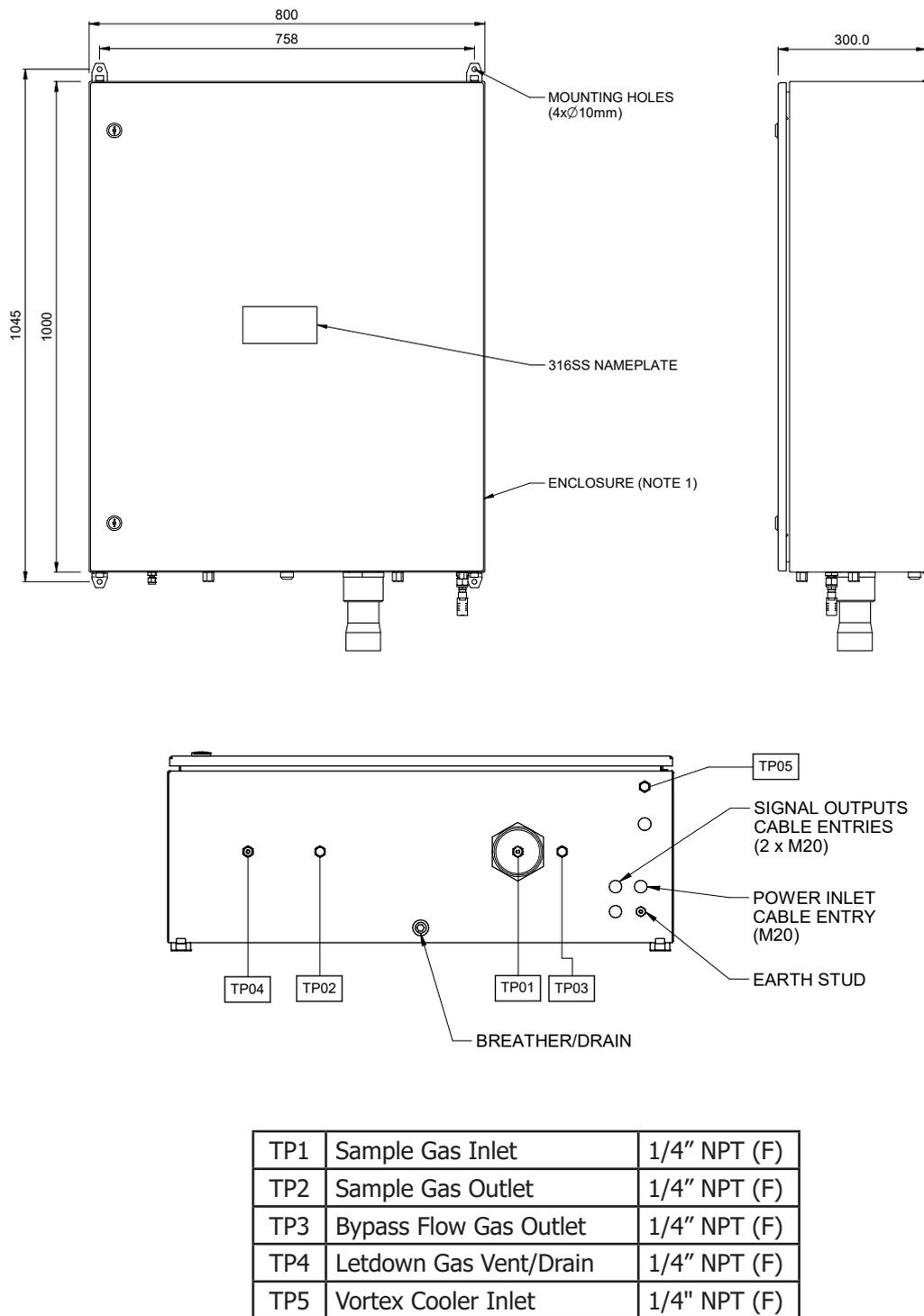
Figure 9 OptiPEAK Sampling System – Typical Outdoor Version
