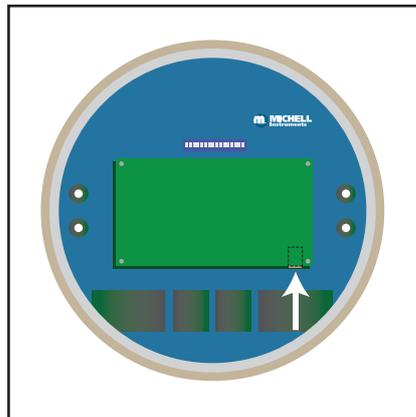
7. Reconnect the HMI Data cable and ensure it latches into the socket.
