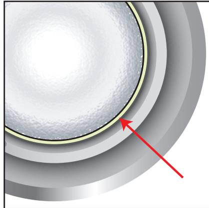
6. Inspect the flame path / threaded joint between the lid and body for damage to the threads.
