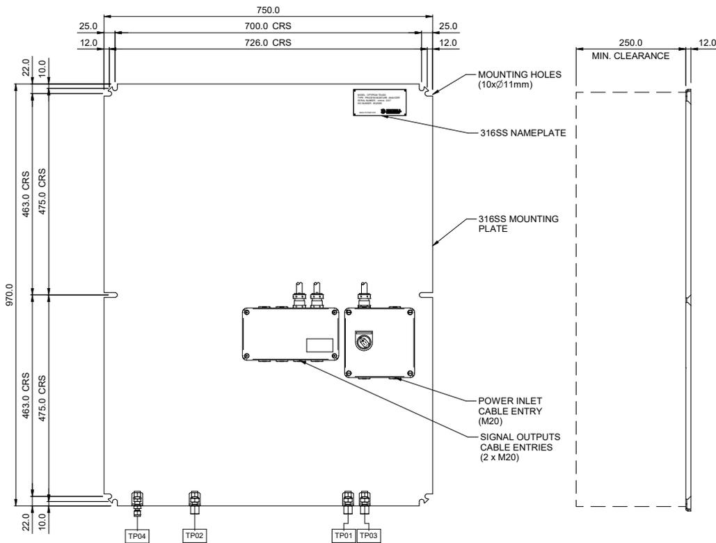
Figure 7 OptiPEAK Sampling System – Typical Indoor Version
