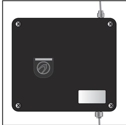
3. Remove the Exd enclosure lid by unscrewing the hex locking screw and turning the lid counter-clockwise until the threads disengage. **CARE SHOULD BE TAKEN AS THE LID WEIGHS IN EXCESS OF 2KG.**
