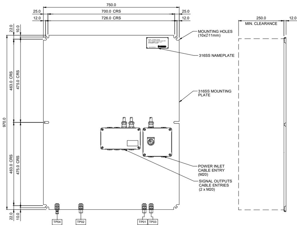
Figure 33 Dimensional Drawing – Indoor System Enclosure
