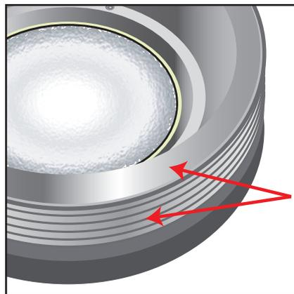
7. Inspect the gasket for pitting, damage or signs of corrosion.
