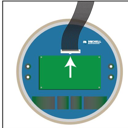
6. The micro SD card, is located on the green, rectangular display PCB, in the bottom right hand corner. It may be necessary to use tweezers or a small pair of pliers when fitting a new micro SD card.
