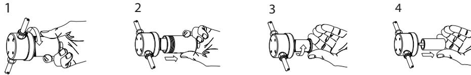
The disposable coalescing filter element is sealed by compression against a flat surface. Gaskets are not required between the filter element and components of the housing. The element is located by guides which fit the inside diameter of the tube at each end. The element is sealed by tightening a threaded element retainer.
