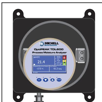
5. Disconnect the display data cable by releasing its latch.
