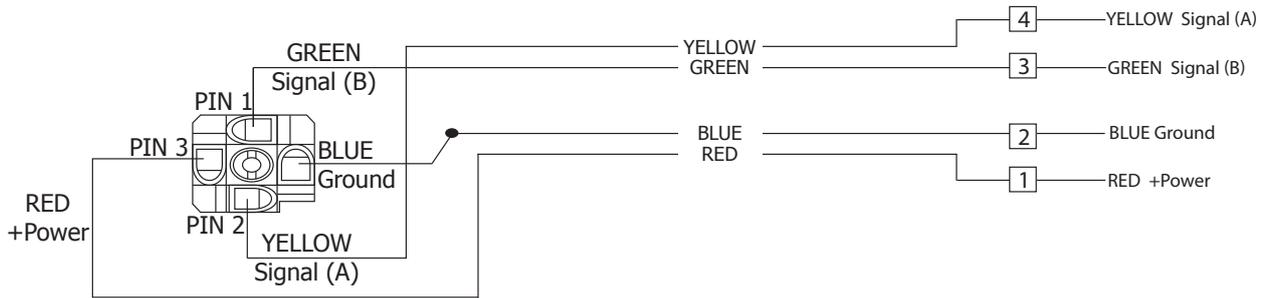
Figure 12 Cable Connections
