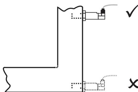
Figure 21 *Installation Location*
