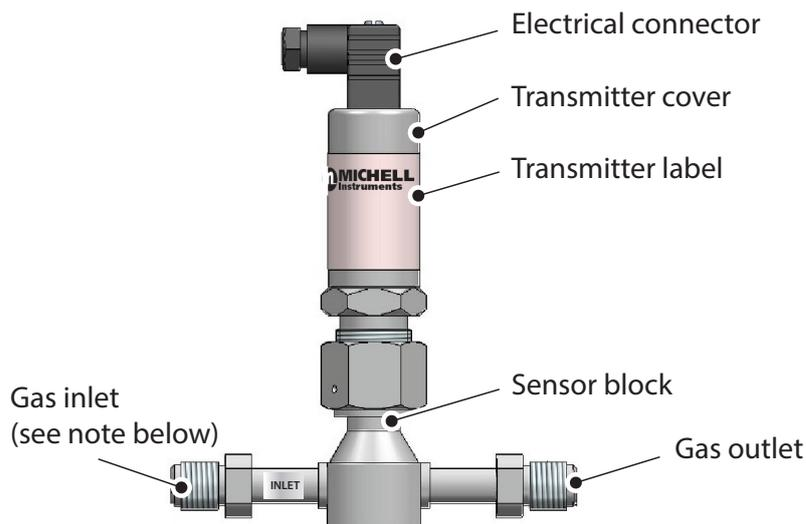
**NOTE:** The Pura has a uni-directional connection and must be connected so the upstream flow is connected to the inlet port of the Pura block (marked with a silver label).
