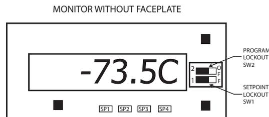
Figure 19 Location of the Lockout switches
