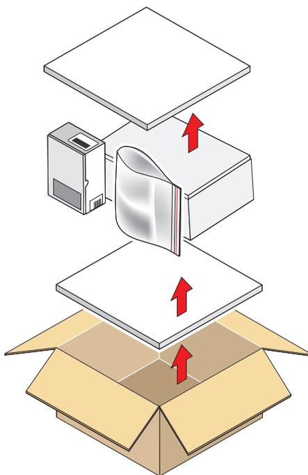
Figure 2      *Unpacking – Monitor and Pura OEM / PRM*
