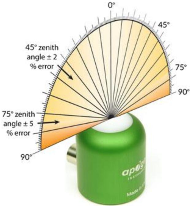
Directional, or cosine, response is defined as the measurement error at a specific angle of radiation incidence. Error for Apogee SE series photometric sensors is approximately ± 2 % and ± 5 % at solar zenith angles of 45° and 75°, respectively.
