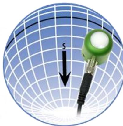
In addition to orienting the cable to point toward the nearest pole, the sensor should also be mounted such that obstructions (e.g., weather station tripod/tower or other instrumentation) do not shade the sensor. **Once mounted, the green cap should be removed from the sensor.** The green cap can be used as a protective covering for the sensor when it is not in use.
