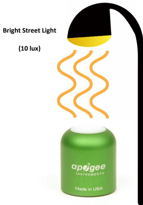
Example of illuminance measurement with an Apogee photometric sensor. Bright streetlights yield an illuminance on a horizontal plane at approximately 10 lux. This yields an output signal of 10 mV. The signal is converted to illuminance by multiplying by the calibration factor of 1 lux per mV.
