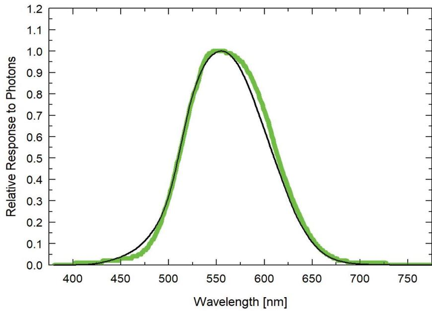
The mean relative spectral response of four SE-100 photometric radiometers (green) compared to CIE-1931 curve (dotted).
