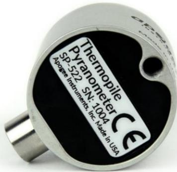
A sensor's model number and serial number are located on the bottom of the sensor. If the manufacturing date of a specific sensor is required, please contact Apogee Instruments with the serial number of the sensor.
