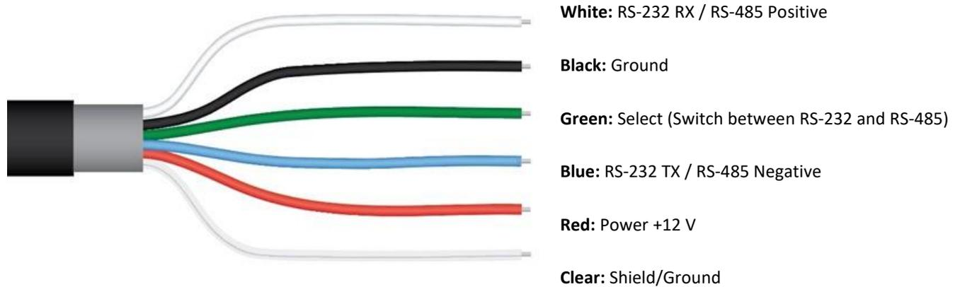
The green wire should be connected to Ground to enable RS-485 communication, or it should be connected to 12 V power for RS-232 communication. Text for the White and Blue wires above refers to the port that the wires should be connected to.
