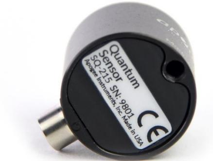
A sensor's model number and serial number are located on the bottom of the sensor. If you need the manufacturing date of your sensor, please contact Apogee Instruments with the serial number of your sensor.
