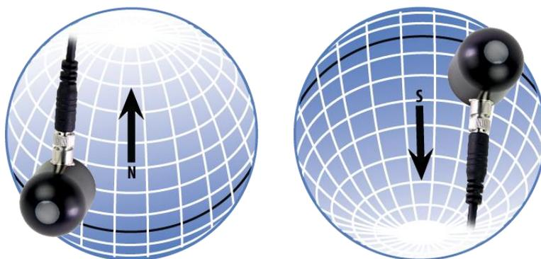
In addition to orienting the cable to point toward the nearest pole, the sensor should also be mounted such that obstructions (e.g., weather station tripod/tower or other instrumentation) do not shade the sensor. **Once mounted, the blue cap should be removed from the sensor.** The green cap can be used as a protective covering for the sensor when it is not in use.
