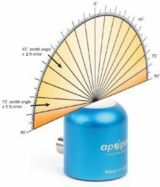
Directional (cosine) response is defined as the measurement error at a specific angle of radiation incidence. Error for Apogee SQ-500 series quantum sensors is approximately  $\pm 2\%$  and  $\pm 5\%$  at solar zenith angles of  $45^\circ$  and  $75^\circ$ , respectively.
