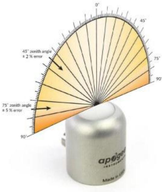
Directional, or cosine, response is defined as the measurement error at a specific angle of radiation incidence. Error for Apogee SQ-600 series Quantum Light Pollution Sensor is approximately  $\pm 2\%$  and  $\pm 5\%$  at solar zenith angles of  $45^\circ$  and  $75^\circ$ , respectively.
