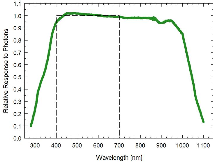
Mean spectral response measurements of six replicate Apogee SQ-600 series Quantum Light Pollution Sensors. Spectral response measurements were made at 10 nm increments across a wavelength range of 300 to 1100 nm in a monochromator with an attached electric light source. Measured spectral data from each quantum light pollution sensor were normalized by the measured spectral response of the monochromator/electric light combination, which was measured with a spectroradiometer
