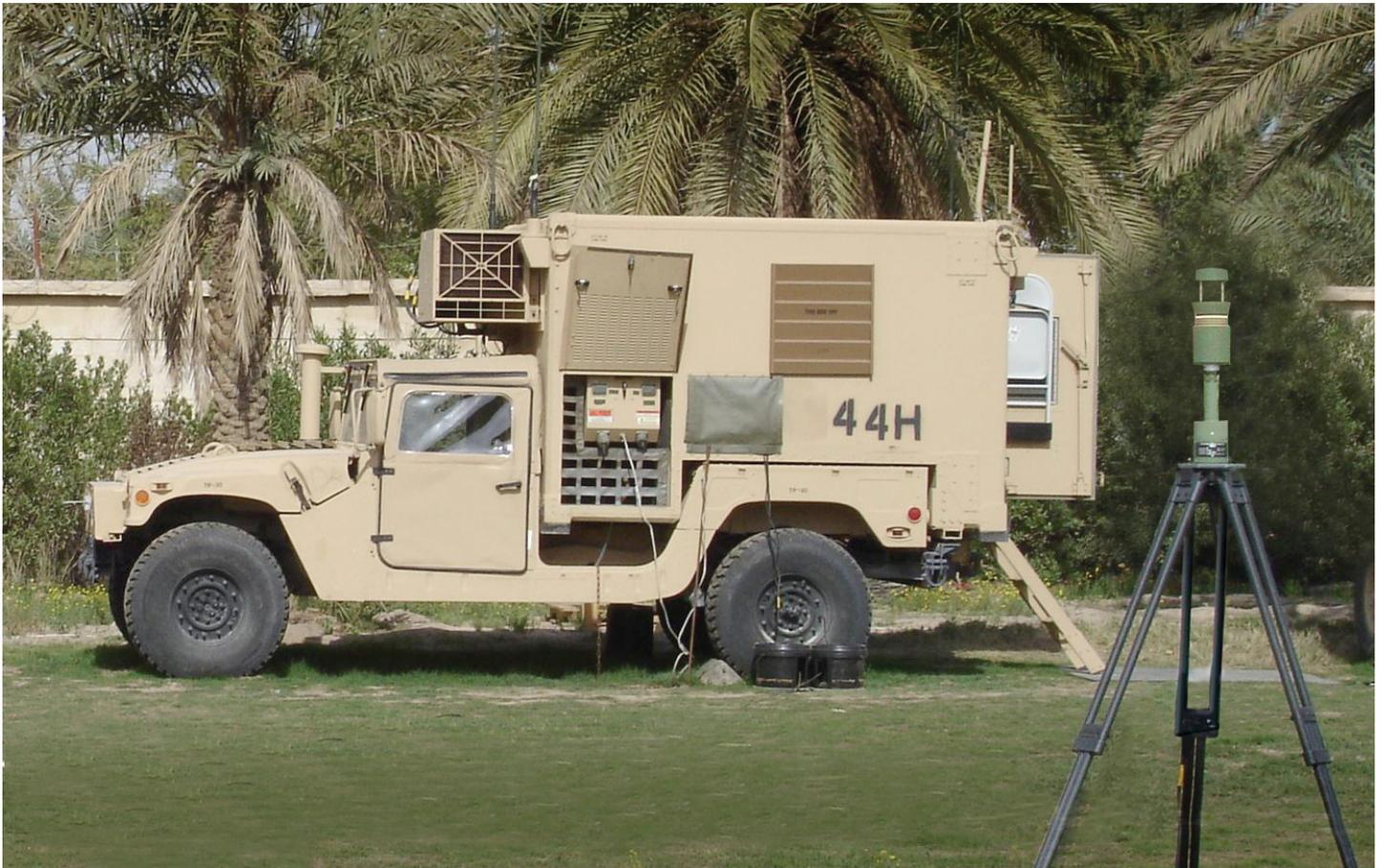
**Met One Instruments' TACMET II Weather Sensor (EMI)** is a second-generation weather sensor, which includes a number of features now possible with new sensor technology as a result from our commitment to product improvement. The TACMET II (EMI) incorporates Met One's new and unique folded-path, low-power sonic anemometer, the Sonimometer, with temperature sensor, a fast-response capacitive relative humidity sensor, and a flux-gate compass. An on-board microprocessor provides a digital output
