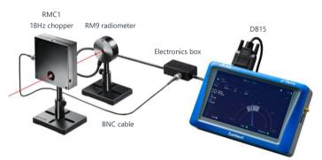
The RMC1 chopper should be mounted with the side marked "THIS SIDE TOWARD SENSOR" facing the RM9. The side of the chopper blade facing this direction has a low emissivity surface to minimize measurement artifacts that could be caused by thermal signal from the chopper blade. The other side of the blade faces the light source and has an absorptive black coating to minimize stray reflections.
