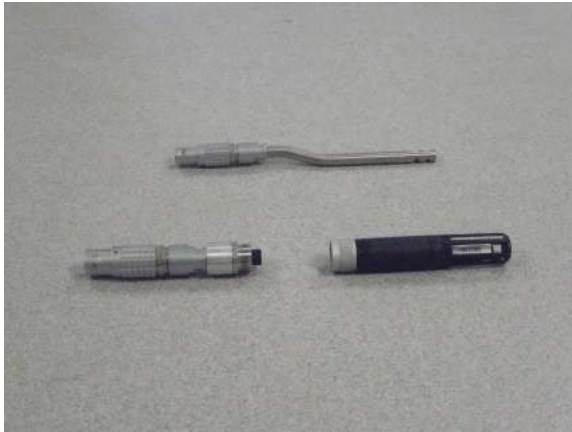
Figure 45: Control PT100 and HC2 separated from Lemo housing
