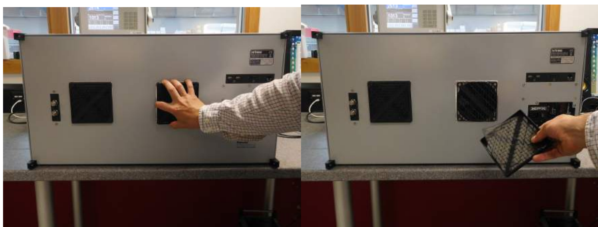
Figure 47: HG2-XL Air inlet filter removal
