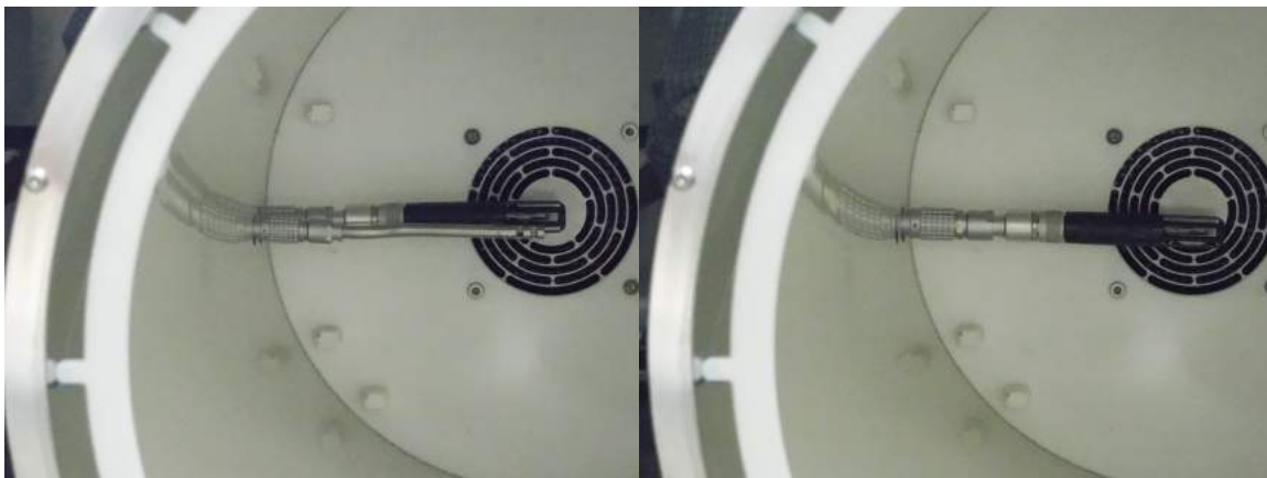
Figure 44: HG2-XL Control HC2 and PT100 Sensor, and with latter removed
